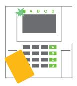
Authorize yourself using the keypad. Function buttons A, B, C, D will light up and the system indicator starts flashing green.
