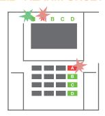
1. When you enter the building (triggering a detector with a "Delayed zone" reaction), the system starts indicating an entrance delay with a continuous tone, the system indicator and a function button, both flashing red, of the section in which the delayed entrance has been triggered.
