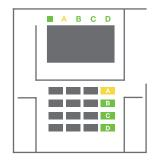
3. The command is executed and the function button turns permanently yellow to indicate a partially set section.
