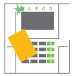
Authorize yourself using the keypad (enter a code or hold an RFID card or tag up to the reader). The system indicator button will start flashing green.
