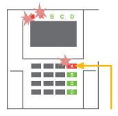
2. Press the function button of the section in which the alarm has been triggered.
