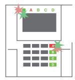
3. Unsetting is finished and sirens are silenced. Rapidly alternately flashing function buttons (green/red) and the status indicators indicate the alarm memory.
